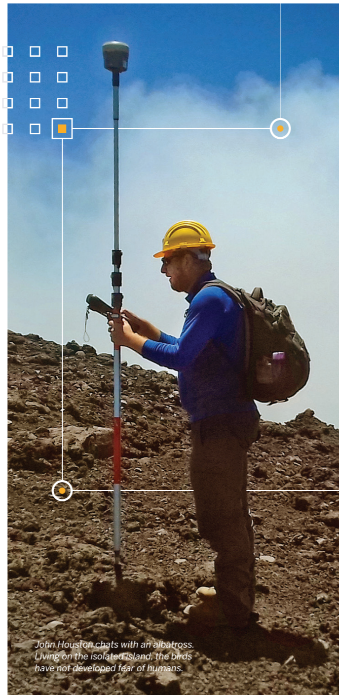
John Houston places the GNSS receiver along a survey line on Gough Island. Cold weather and difficult terrain made days difficult.
